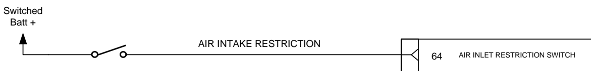
Figure 13.2 Air Intake Restriction Switch Installation wiring
